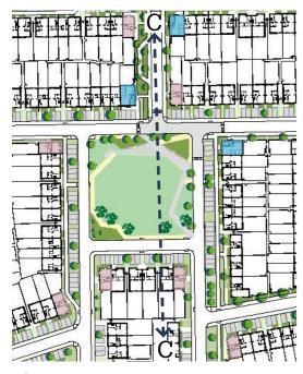
Part Plan with 3 storey duplex units highlighted in blue & 2 storey dual frontage houses highlighted in pink holding and aminating the corners of streets.
