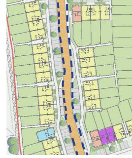
Neighbourhood street which offers a variety of parallel & perpindicular street parking for residents and suitable landscape in between A mix of car parking arrangements are provided within the scheme to reflect the varied nature of the proposed housing & duplex units. A minimum of 2 no. car parking spaces on curtilage per house are provided and one space for the narrow frontage 2 bedroom houses on curtilage, and a number of visitor spaces on streets nearby.
