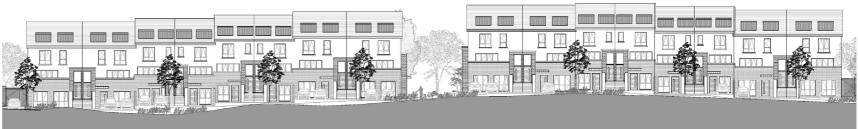
A Three Storey stepped facades with selected brick to the lower bays, and lower gable returns. Elevation & street frontage is further animated with patio and terraces to ground & first floor levels.
