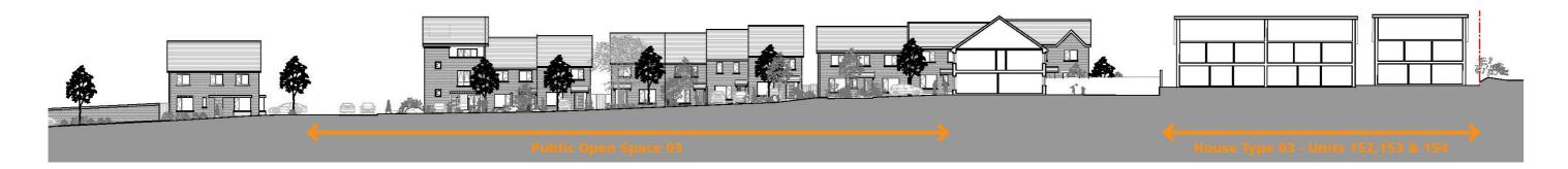
Part section CC - 2 storey terrace houses with Duplex corner unit overlooking POS 03. No overlooking from House Type 03 at first floor to the rear of their properties. Note, rear access is provied for all units to back gardens for private access & bin storage
