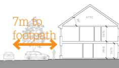
Typical section of 2 storey traditional house with level access & on curtilage parking
